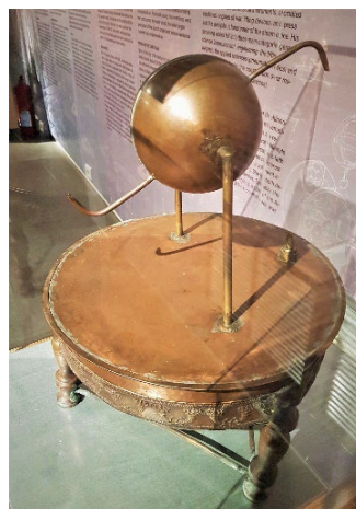
Heron's engine, the aeolipile Credit: Wikimedia Commons
